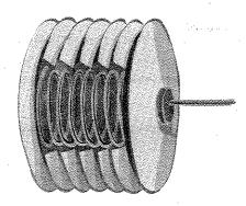
If the atmospheric pressure increases, it will push on the bellows. The ends of the bellows will be pushed closer together until the force pushing back by the spring is equal to the increased air pressure. A pointer attached to the bellows moves along a scale to show the change in pressure.
