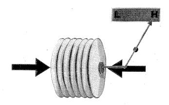
Lower pressure allows the spring inside the bellows to push the ends of the bellows farther apart.
