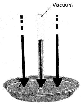
What was holding the heavy column of mercury up in the tube? Atmospheric pressure. Air pressure pushes down on the mercury in the dish. The pressure is distributed throughout the mercury, including the mercury in the tube. Remember, a column of atmosphere 1 cm² has a mass of 1.2 kg. If the column of mercury is 1 cm² in cross section, it will have a mass of...that's right, 1.2 kg. So, the air pressure is exactly balanced by the mercury pressure.
