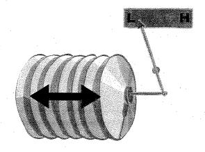
Sometimes a pen is attached to the bellows. The pen records the air pressure on a rotating cylinder to obtain a continuous record of pressure changes. If an electronic sensor and a transmitter are attached to a barometer, pressure information can be radioed from a weather balloon back to a receiving unit on Earth.
